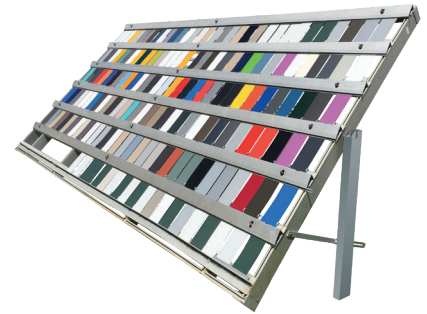
Outdoor testing rack with painted panels
