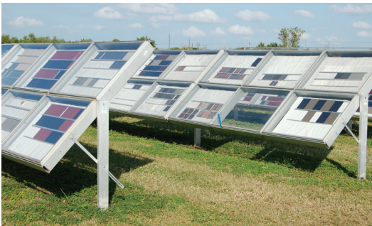
Under Glass Exposures are used to test interior materials such as textiles and printed materials
