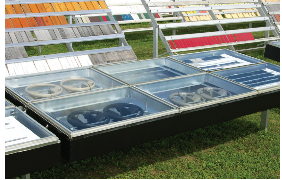
Black Box Exposures are designed to simulate automotive conditions
